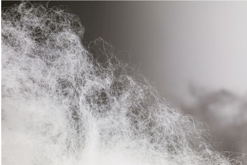
Caption: New PET-core-BICO Fibres for resilient, high loft hygiene nonwovens. (Photo: © Beaulieu International Group)
