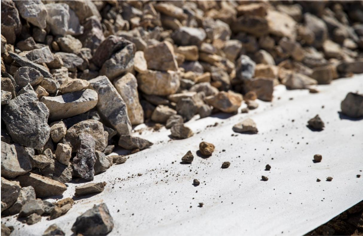
*Caption: Fibres for lightweight high-performance nonwoven geotextiles.*
